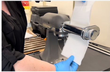
Membrane casting Scale up from 2 by 2-inch to 4 by 8-inch
